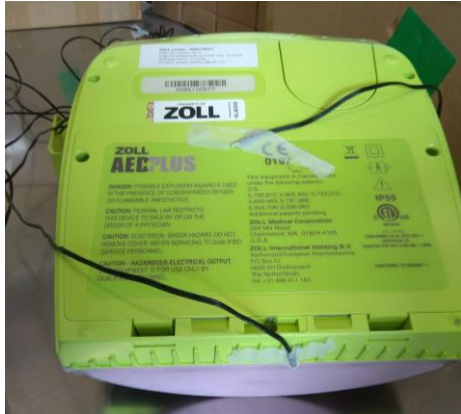
Figure 2-4: Temperature probe 3 and 4: At the back and bottom of the AED
