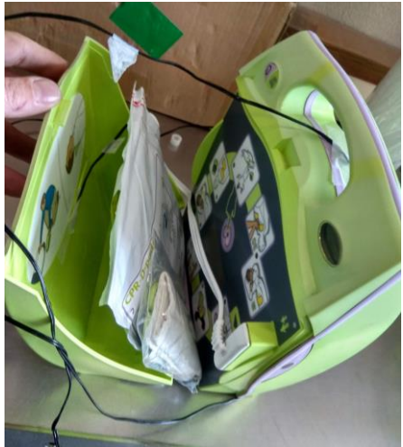
Figure 2-3: Temperature probe 2: top of the AED
