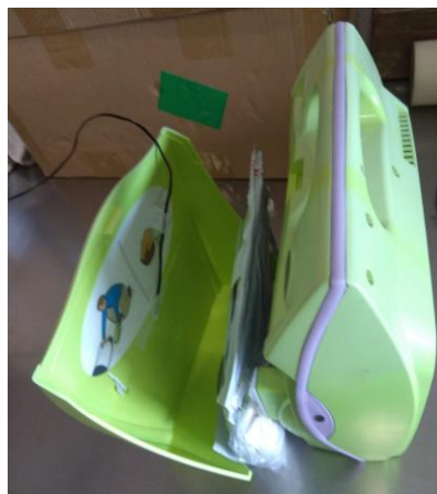
Figure 2-2: Temperature probe 1: in front of the AED pads
